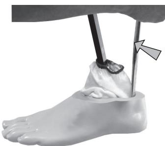
Using a lever, ease assembly into shell.
